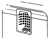
The Air Freshener Compartment is designed to help control odors that might develop in the trash. There are many solid air fresheners available on the market.
